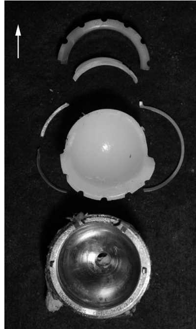
Figure 2-4 - Example of a retrieved fractured remelted HXLPE liner at the implant rim. (Permissions from Moore KD, Beck PR, Petersen DW, Cuckler JM, Lemons JE, Eberhardt AW. Early Failure of a Cross-Linked Polyethylene Acetabular Liner: A Case Report. J Bone Joint Surg Am. 2008;90(11):2499-2504. doi:10.2106/JBJS.G.01304)
